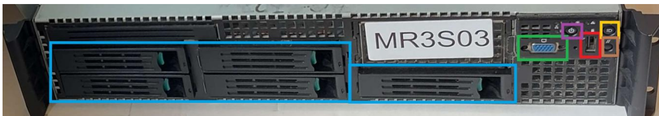
2 Front panel — drive bays and control buttons
